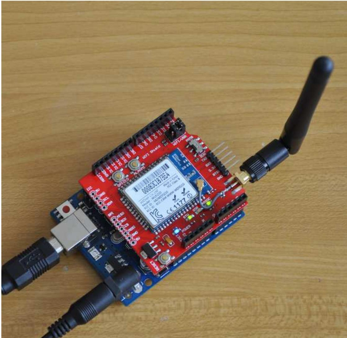
Now open a terminal. You can use PuTTY, or if you have a Windows XP machine you can use the Hyperterminal included. and connect to the WiFi shield's IP address. Don't forget to indicate the server port. In our example we are using port "4000".
